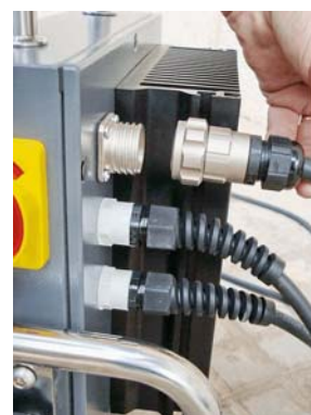
Figure 11b: Mains cable (unplugged)
