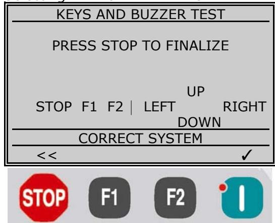
This option allows you to check the performance of all the buttons (arrows, keys STOP, F1, F2, VALIDATE) and the buzzer. Each press the key pressed together with the acoustic signal is displayed.
