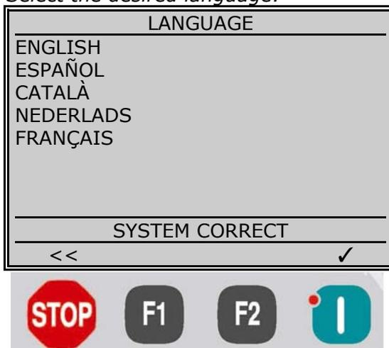
Now select the desired language by placing the cursor on the chosen one using the arrows **↑** and **↓** on the panel. Then press <VALIDATE> to validate command.
