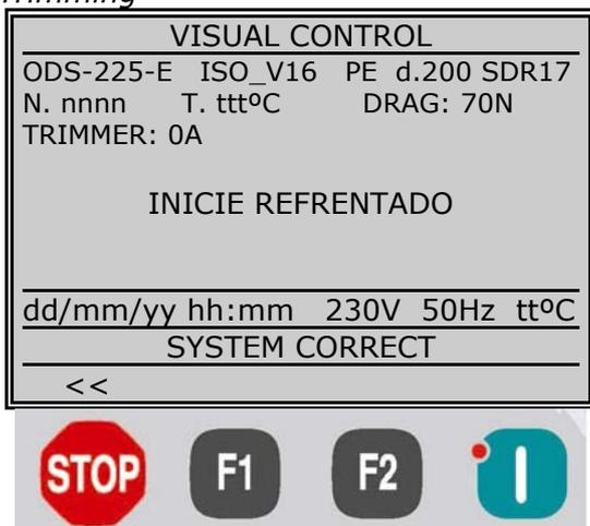
**NOTE:** For electrically operated machines (**ODS225E**), be sure that the trimmer is properly setup:
