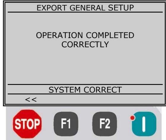
Connect a memory stick (FAT or FAT32) in the connector USB/A (located on the left side of the unit).
