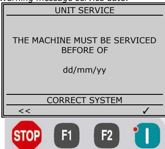
If the date **dd/mm/yy** has not yet passed the service date or having expired, the unit is set without lock, press the VALIDATE button and move to the next screen work. However, if the date **dd/mm/yy** has expired but the unit is configured to lock the box, it can not be used until has not made the annual service.
