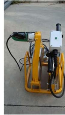
Figure 7b: Heating plate and trimmer holder
