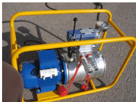
Figure 8a: hydraulic station at 230 Vac
