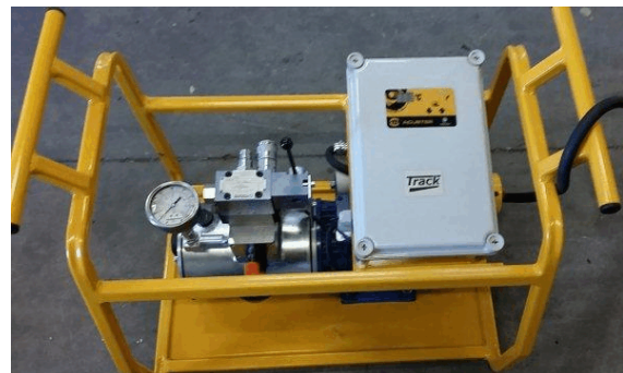
Figure 7b: hydraulic station at 400 Vac
