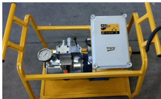
Figure 8b: hydraulic station at 400 Vac
